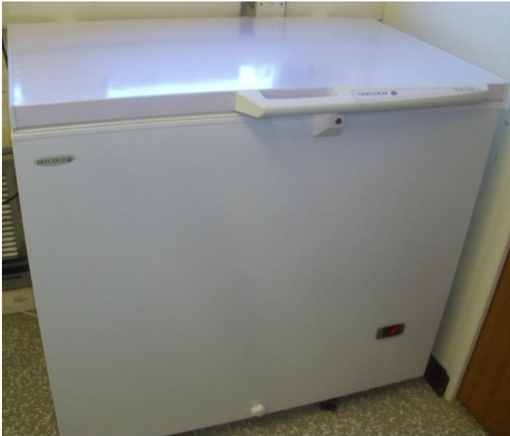
Figure 3.1: Tefcold freezer in the Laser Ablation Laboratory at Royal Holloway University of London. Operating temperature range from -36 to -38 °C. The freezer has been plugged into an Uninterrupted Power Supply (UPS) socket.
