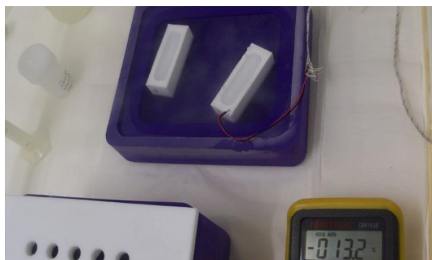
Figure 3.8: Ice Standard preparation. Two different teflon moulds were dipped inside the HDPE coolbox lid. The standard solution was poured in different steps inside the moulds. As soon as the solution was poured shock freezing took place. This procedure avoids redistribution of elements in the ice caused by the process of freezing. The less the quantity of solution is poured in every step, the faster the freezing it is, and thus the less inhomogeneous the ice standard it is. However, PTFE surface do not allow a sufficient spreading of liquid and thus results in inhomogeneity. The temperature of the mould was constantly monitored. On average: -13.2 °C on the outer side, -101.7 °C on the bottom of the mould.
