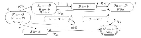
Recall that the RIGLR recogniser uses sets  $P_i$  to record RCG nodes, constructed at the current step, that have been popped. In the parser version we need the SPPF contexts associated with the pops in order to construct the new SPPF node. Thus  $P_i$  is a set of pairs (q, L) where q is an RCG node and L is a set of SPPF nodes which are the contexts in which q has been popped.
