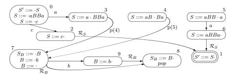
We begin by creating an RCG node  $q_0$  labelled -1 and a descriptor  $(0, q_o, null)$  that we add to  $U_0$ . The first input symbol is a and the RCAstate 0 has an a-transition to state 3. Thus we create an SPPF node  $w_1$  labelled (a, 0, 1) and add  $(3, q_0, w_1)$  to  $U_1$ . All the descriptors in  $U_0$  have now been processed so Step 0 is complete.
