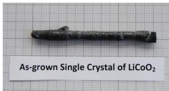
Figure 1: As-grown single crystal of \text{Li}_{0.87}\text{CoO}_2
