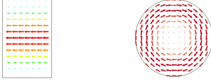
Figure 2.3: The electric field and magnetic fields for a \text{TM}_{010} mode in a pillbox cavity.
