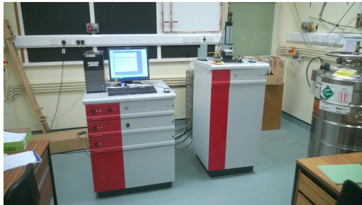
Figure 3.4: The 7 tesla SQUID magnetometer at the Clarendon Laboratory in Oxford. –
