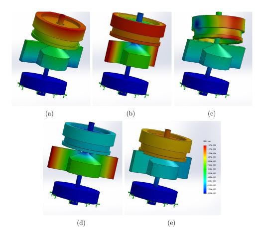
Figure 4.10: CAD software simulation of some of the resonant modes of the oscillator. In order of increasing frequency, a low frequency floppy mode (a), the symmetric torsion mode (b), a high frequency floppy mode (c), the antisymmetric torsion mode (d), and a very high frequency stretching mode (e). Displacement from the stationary position is shown as a colour gradient from blue to red.
