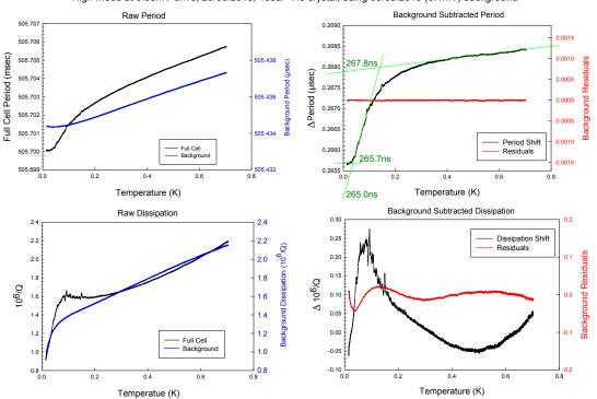
High mode at 0.05mV drive, 20/06/2013, 43bar  $^4\text{He}$  crystal, using 05/05/2013 (0.1mV) background
