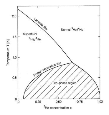
Figure 3.3: The phase diagram of liquid  ${}^{3}\text{He}/{}^{4}\text{He}$  mixtures at saturated vapour pressure. Note the suppression of the superfluid transition, the phase separation of the mixture below 0.8 K and the finite solubility of  ${}^{3}\text{He}$  in  ${}^{4}\text{He}$  at  $T \rightarrow 0$  K. Taken from Pobell [74].
