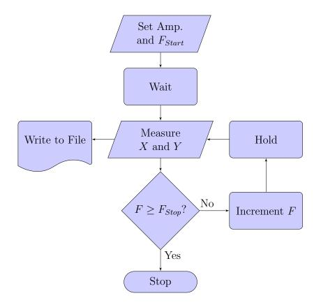
Figure 4.1: Operation schematic of the Frequency Sweeper LabVIEW vi.
