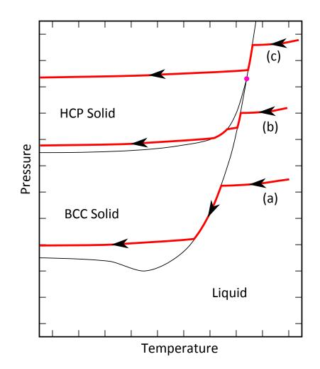
Figure 7.1: Phase diagram of <sup>3</sup>He showing possible blocked-capillary sample growth isochors, (a) BCC throughout, (b) HCP cooled through BCC, and (c) HCP throughout. The tri-critical point is shown in pink.
