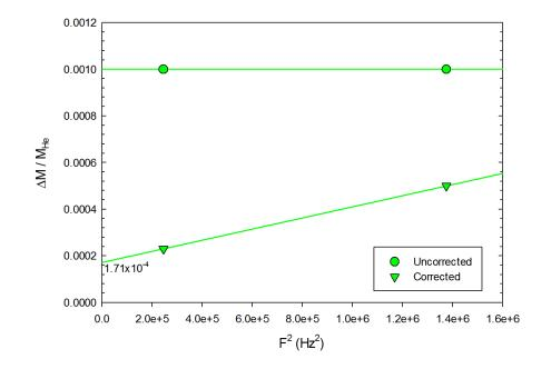
Figure 6.3: Data of Aoki *et al*, original (circles), and with shear modulus correction applied (triangles).
