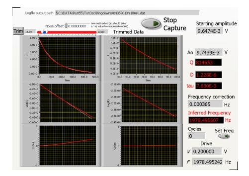
Figure 4.5: A captured ringdown. Note the deviation from an exponential in the untrimmed (left) plots.
