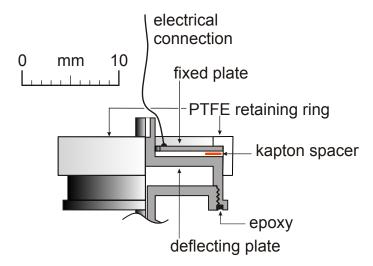
Figure 2.9: The pressure gauge assembly.
