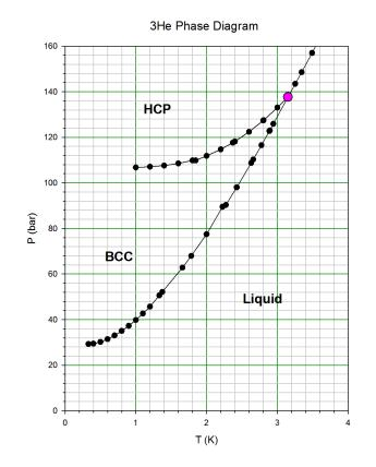
Figure 5.7: The P - T phase diagram of <sup>3</sup>He. The tri-critical point at 3.148 K and 137.7 bar is shown in pink. Data taken from Straty and Adams [84], and Grilly and Mills [38]
