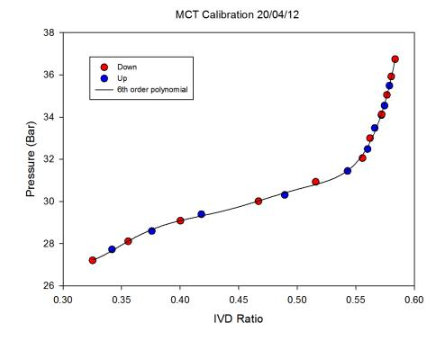
Figure 3.5: A calibration curve of the original MCT showing the poor stress-strain relationship. The cell has poor sensitivity at higher pressures, and shows significant hysteresis between raising (blue points) and lowering (red points) the pressure. A  $6^{\text{th}}$  order polynomial is fitted to the calibration sweeps.
