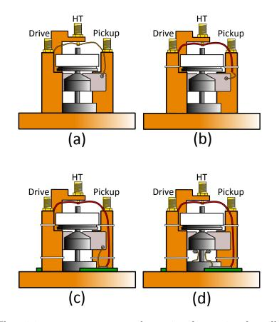
Figure 2.8: The wiring arrangements used to raise the torsional oscillator vanes to high voltage. Directly from the connector, (a), via a thicker wire secured to the posts, (b), via a PCB pad (green), (c), and to a tab on the vanes, (d).
