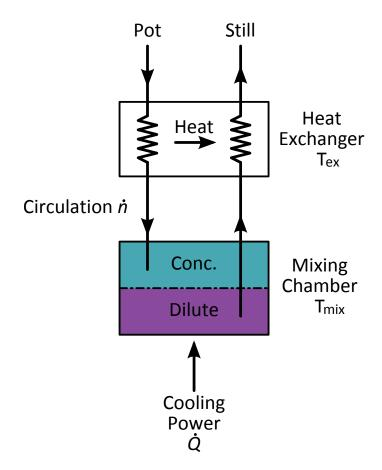
Figure 3.4: Heat flow in the dilution unit.
