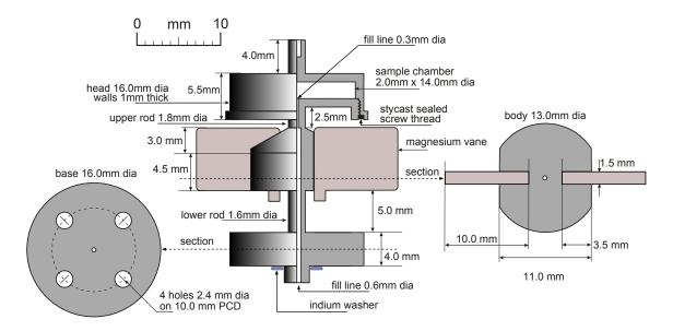
Figure 2.7: Technical drawing of the torsional oscillator cell. The pressure gauge assembly is shown separately in Fig. 2.9.
