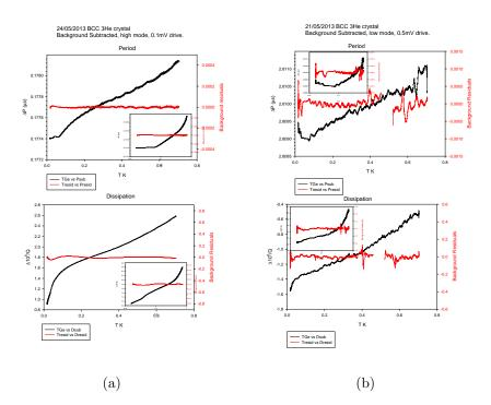
Figure 5.8: Behaviour of the <sup>3</sup>He sample at high frequency (a) and low frequency (b). Empty cell background behaviour has been subtracted. The errors from the background fitting are shown in red. Period shift is shown at the top and dissipation at the bottom.
