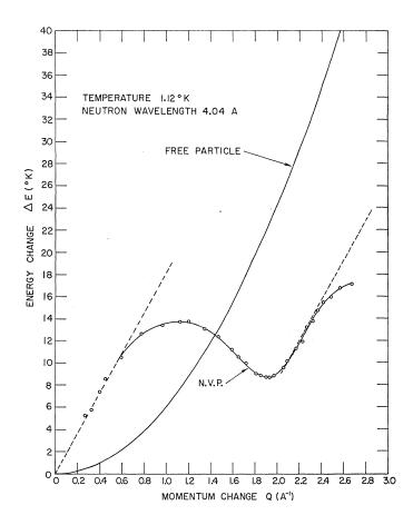
Figure 1.4: The excitation spectrum of liquid <sup>4</sup>He, measured by neutron scattering, confirming the roton minimum proposed by Landau. [42].
