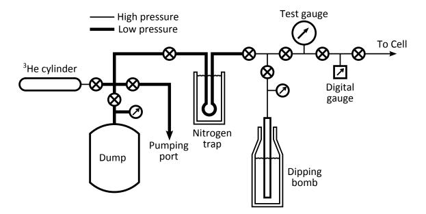
Figure 5.1: The sample gas handling system.
