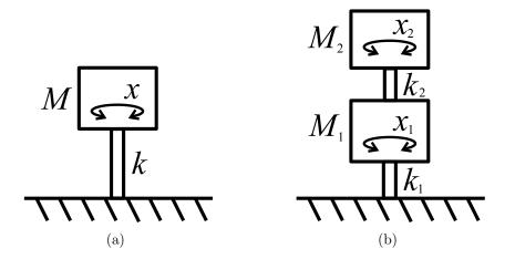
Figure 2.5: A single (a) and double (b) torsional oscillator.
