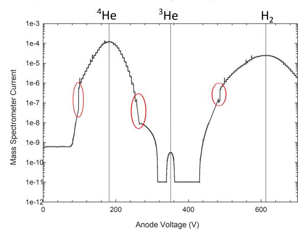
Figure 5.16: Mass spectrometry of the <sup>4</sup>He sample. The isotope peaks are labelled along the top edge. The discontinuous features circled in red are artefacts from the leak detector automatically changing its preamplifier gain.
