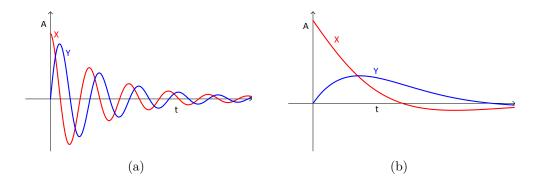
Figure 4.6: The symmetric and antisymmetric signals during ringdown from well off resonance (a) and near resonance (b) showing the phase progression. A ringdown from exactly on resonance would have zero Y component and be entirely exponential in X.
