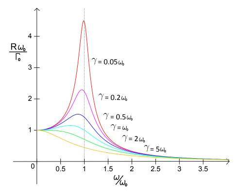
Figure 2.4: The steady-state response of a forced harmonic oscillator with different amounts of damping. As the damping is decreased the resonance better approximates a Lorentzian peak and the peak position approaches  $\omega_0$ .
