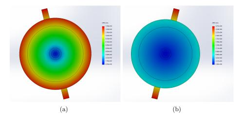
Figure 4.11: Plan view of the two torsion modes. (a) shows the symmetric, low frequency mode and (b) shows the antisymmetric, high frequency mode.
