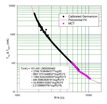
Figure 3.7: Generic calibration applied to all  $\text{RuO}_2$  resistors. The MCT (pink data points) is used at temperatures below the limit of the germanium thermometer (black data points). In the vicinity of the melting curve minimum the MCT becomes insensitive, so the germanium is used for higher temperatures.
