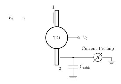
Figure 2.3: Top-down schematic of the electrical contacts of torsional oscillator, showing the capacitatively coupled electrodes.
