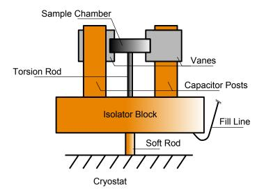
Figure 2.2: A schematic diagram of a modern torsional oscillator.
