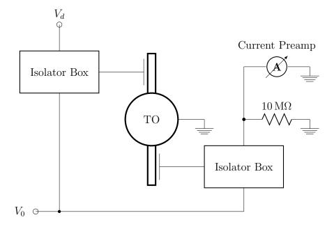
Figure 2.10: A schematic of the torsional oscillator connected in 'grounded' mode. The electrode posts are raised to high-tension  $V_0$  and the oscillator vanes are grounded. The isolator boxes contain the circuit shown in Fig. 2.11 to add the AC signal on to the DC drive while keeping the instruments isolated from high voltages. A 10 M $\Omega$  shunt resistor is added to the input of the current preamp to dissipate any residual charge when it is switched off.
