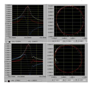
Figure 4.4: Sweeping through the resonance slightly too fast (top) and much too fast (bottom). The distortion of the peak, top left, is slight but clearly visible as a distortion of the circle, top right. Notice that the 'ripples' in the frequency domain, bottom right, appear as loops in the complex plot, bottom right.
