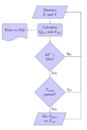
Figure 4.9: Operation schematic of the Temperature Sweeper LabVIEW vi. is losing less energy, and if it is lower the amplitude will be lower.
