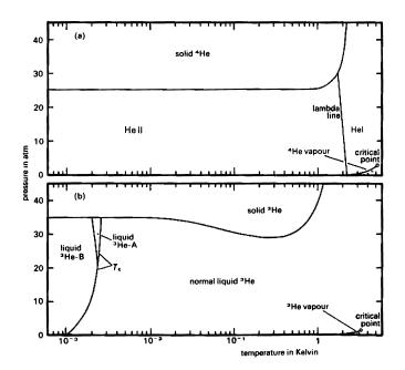
Figure 1.1: P - T phase diagrams of <sup>4</sup>He (a) and <sup>3</sup>He (b).
