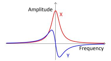
Figure 2.13: The in-phase X and quadrature Y response of the torsional oscillator as measured by two-channel lock-in detection.
