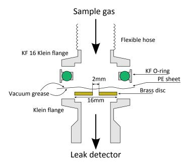
Figure 3.9: Exploded cross section of the control leak used to measure the mash concentraion.
