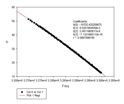
Figure 5.2: Calibrating the cell pressure gauge against the Paroscientific gauge. This plot includes points taken both on increasing and on decreasing the pressure and is fitted with a third order polynomial.
