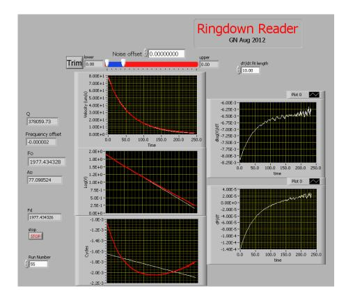
Figure 4.8: A captured ringdown shown in red in the left hand plots. The slopes of  $\ln(R)$  and the phase progression are shown in white in the right hand plots.
