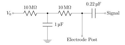
Figure 2.11: The isolator circuit used to superimpose the AC signal onto the high-tension DC at the electrode posts without damaging instrumentation.
