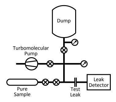
Figure 3.10: The gas handling system used to measure the isotopic composition of the mash.
