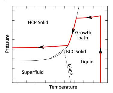
Figure 5.3: Typical blocked capillary growth of a  ${}^{4}$ He sample. The cell is loaded with liquid. It contracts slightly on cooling and joins the melting line and the sample starts to freeze. Because of the difference in density between the solid and liquid phases the mixture follows the melting line until all the liquid is frozen. The solidified sample then leaves the melting line and contracts slightly as it cools.
