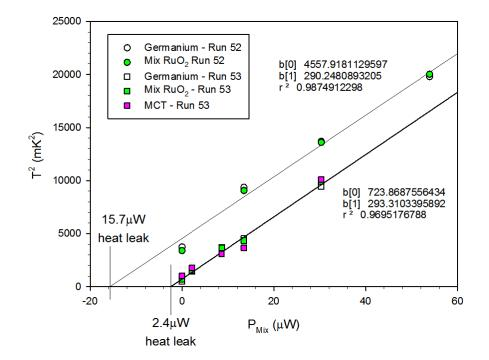
Figure 3.11: Evaluation of cooling performance before (circles) and after (squares) eliminating the heat leak.
