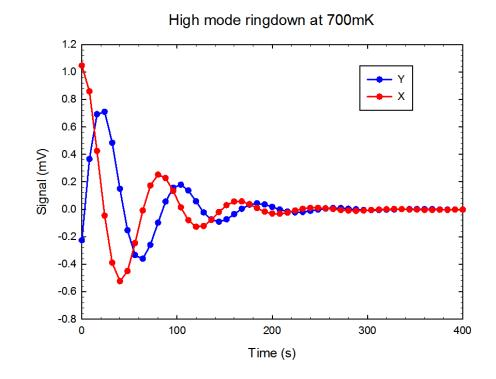
Figure 4.7: A capture of the oscillator's ringdown from some way off the antisymmetric resonance.
