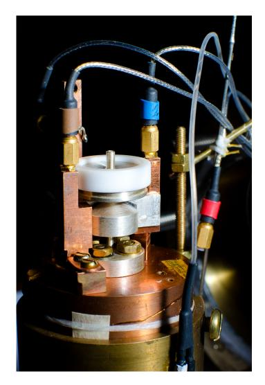
Figure 2.6: The torsional oscillator cell, mounted in a test probe.
