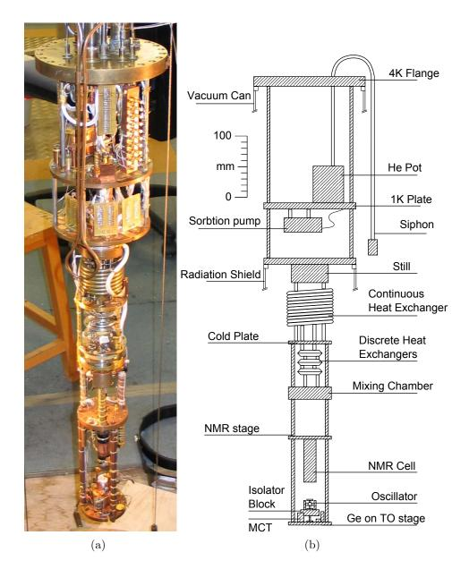
Figure 3.1: The cryostat
