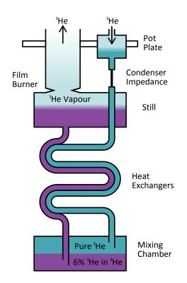
Figure 3.2: Schematic diagram of the dilution unit.
