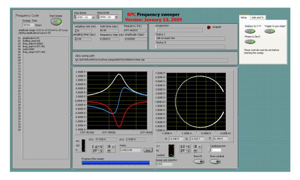
Figure 4.2: The frequency sweeper program front panel. The frequency-domain lineshape is shown in the left plot. The amplitude R is shown in white and the Xand Y outputs of the lock-in are shown in red and blue respectively. The right plot shows the same data represented as a complex plot - the X channel is plotted on the horizontal axis against the Y channel on the vertical. The text box on the left is the command-set for the sweep and the tabbed controls on the right are the SR830 settings.
