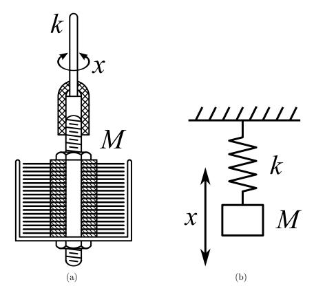
Figure 2.1: A schematic of Andronikashvili's torsion bob oscillator experiment (a) and the mass-spring model (b).
