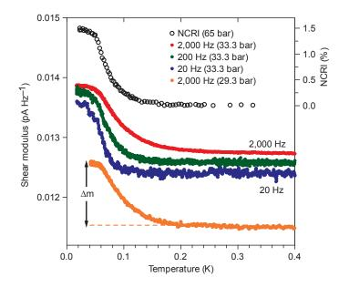
Figure 1.6: Similarity between the torsional oscillator and shear modulus measurements in  ${}^{4}$ He [25].
