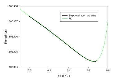
Figure 5.6: Fitting the empty cell background as  $P = a + bt + ct^2 + dt^{13}$  where t = 0.7 - T. The data is black, the fit is overlayed in green.
