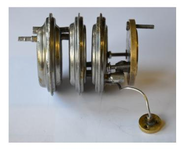
Figure 3.8: The old heat exchanger stack, removed from the cryostat. The two pipes leading into the mixing chamber are on the left. The returning stream leaves through the large flange on the right, joined into the bottom of the cold plate. The condensing stream enters the exchangers through the small flange, bottom right. Note the reflowed solder join on the left-most exchanger.
