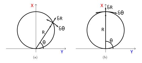
Figure 4.3: The resonance represented as a complex plot. In (a) the drive is off resonance, and in (b) the drive is at the resonant frequency.
