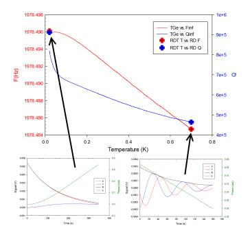
Figure 5.9: The raw f and Q data collected from a twelve hour temperature sweep of the empty oscillator. The smaller plots below show the ringdowns used to collect the initial f and Q parameters used to track the resonance, left, and to remeasure then to confirm that the sweep tracked correctly, right. The small discrepancy at the low temperature (left) end of the sweep is due to the cryostat cooling further after the sweep is completed.
