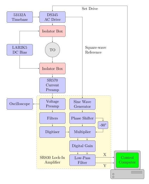
Figure 2.12: The main components of the tosional oscillator instrumentation used in this experiment.
