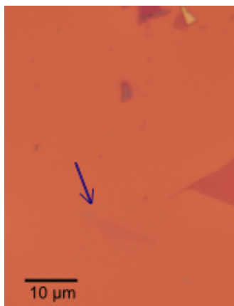
Figure 3.5: Optical image of a graphene flake exfoliated from Kish graphite with a measured contrast of 5% against the substrate background. The flake was confirmed to be monolayer graphene by Raman spectroscopy.
