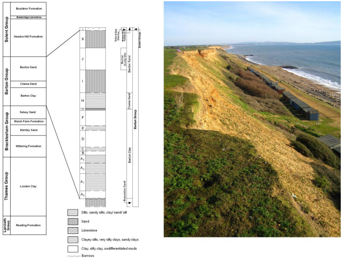
Figure 6.12. Generalised lithostratigraphic succession of the Barton Group, Barton (after Daley, 1999) and slumped cliff exposures of Barton section.
