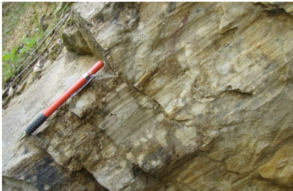
Fig. 60: Typical outcrop of a slickenside with calcite slickenfibres Pen indicates movement direction of the missing block. Outcrop 267, sample KMR-LIV32 in situ before recovery. View towards W.
