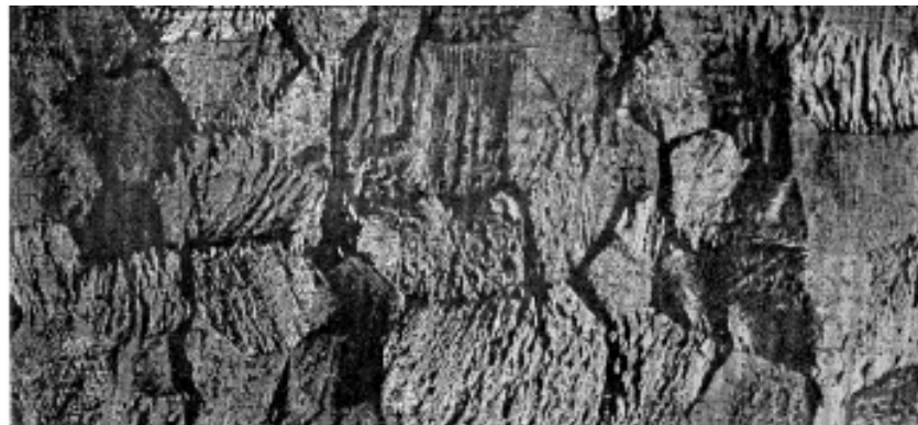
Figure 2.1: Image highlighting large grain domain formation on an iron based sample using the Bitter technique with a magnification of approximately x2
