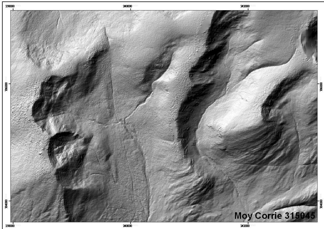
Figure 3.5 Example of relief shading image using the default illumination direction and elevation (Azimuth: 315° , Elevation 45°) settings in GIS. The Location of this image is in the Moy Corrie area at the eastern side of Glen Roy northwestern Highlands, Scotland as shown in Figure 3.4A.
